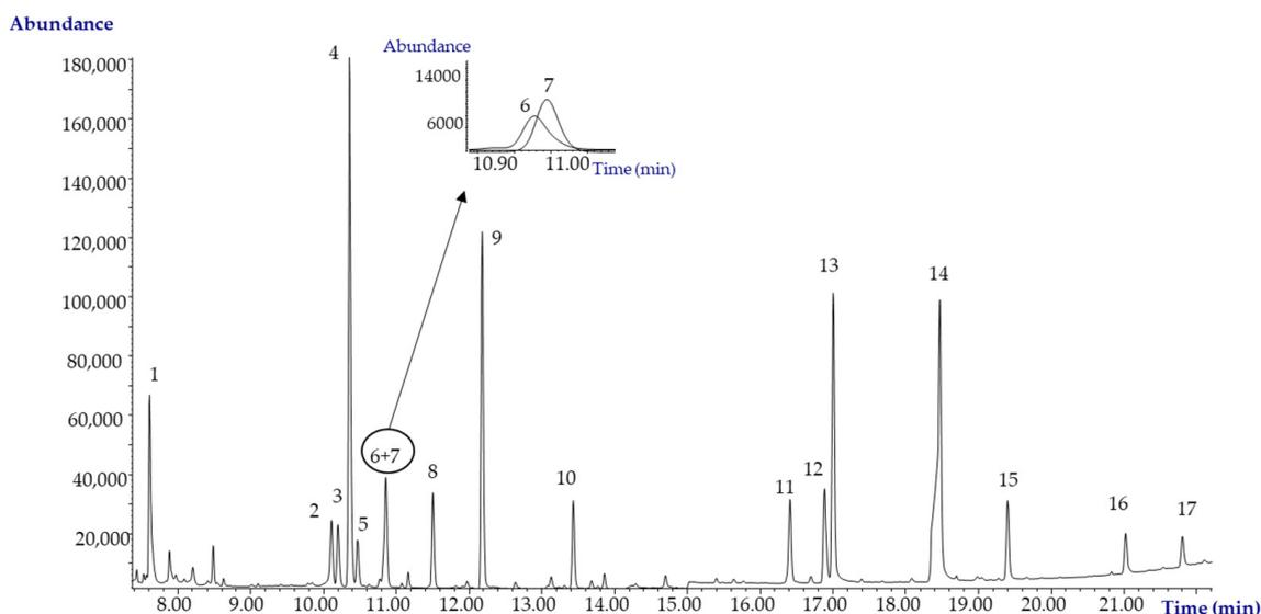
**Figure 2.** Total ion chromatogram (TIC) for a standard solution containing the 17 target compounds at  $1 \mu\text{g mL}^{-1}$  prepared in methanol. Codes: 1: EGDME; 2: EGME; 3: PGME; 4: PGMEA; 5: EGEE; 6: iPGMEA; 7: EGMEA; 8: EGEEA; 9: DEGDME; 10: EGBE; 11: DEGME; 12: DEGEE; 13: ETG; 14: TEGDME; 15: DEGBE; 16: TMG; 17: DEG.
