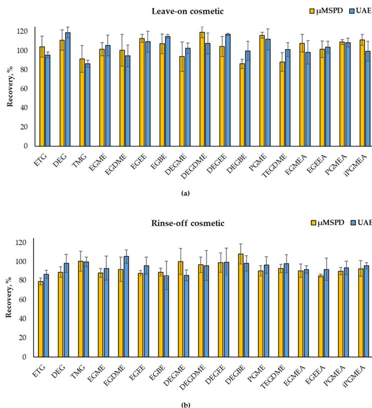
**Figure 3.** Individual recovery values (%) for the UAE- and  $\mu$ MSPD-GC-MS methodologies for: (a) leave-on and (b) rinse off cosmetics samples.
