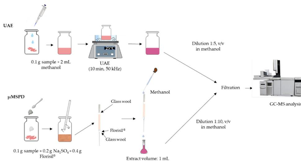
**Figure 1.** Schematic representation of the UAE and µMSPD experimental procedures.
