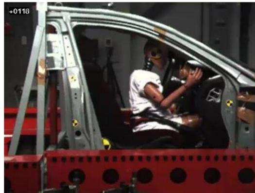
**Figure 2.** Instant at which the chest of the dummy made contact with the center of the steering wheel in test 1.
