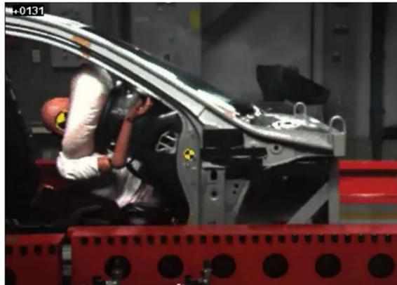
**Figure 5.** Instant at which the entire dummy's torso slid under the instrument panel in test 3.
