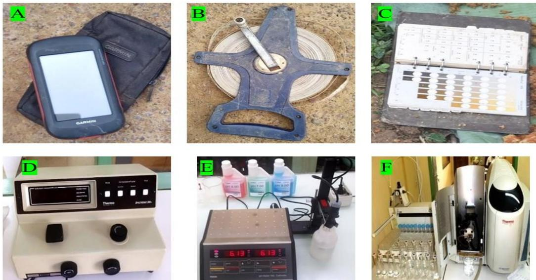
Fig. 2. Soil prospecting and laboratory equipment. A: GPS, B: Tape measure, C: Munsel code, D: Spectrocolorimeter, E: pH meter, F: Spectrometer
