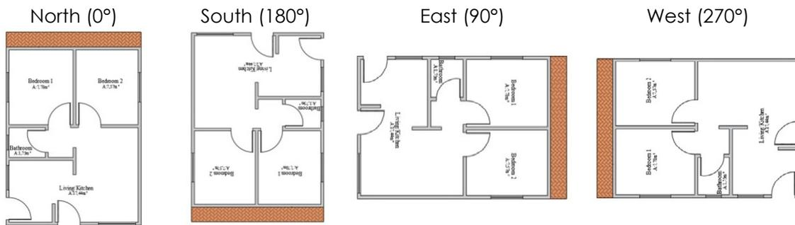
**Figure 4.** Variation of the embedded earth-sheltered wall orientation.
